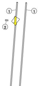
B. Slide the bumpers, weight plates, and top plate assembly down the guide rods.
