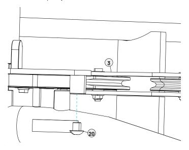
M. Route the main frame cable around the pulleys and pulley cam and fasten it into place.
