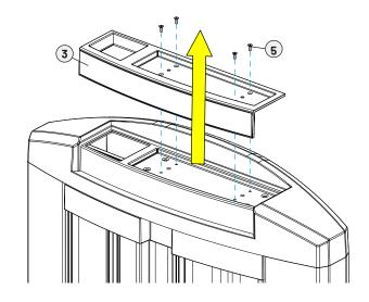
D. Attach the top cover to the upright assembly using the 4 previously set aside top cover hex screws.
