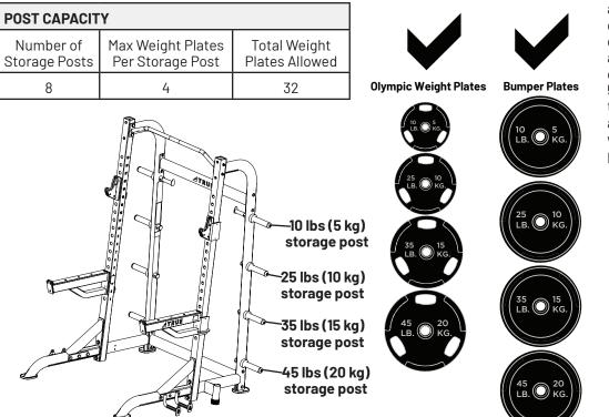
**IMPORTANT!** Storage posts are 50 mm in diameter, designed to accommodate olympic weight plates and bumper plates with center hole diameters of 50 mm. Spacing between the storage posts will accommodate both olympic weight plates and bumper plates.
