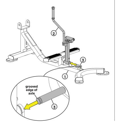
C. Using a 5/32" allen wrench, attach the support arm assembly to the main frame assembly using 1 hex screw, 1 lock washer, and 1 flat washer.
