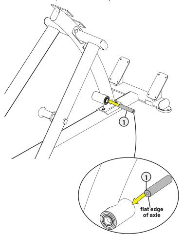
C. Using a 5/16" allen wrench, attach the lever arm assembly to the bottom of the pad frame assembly using 2 hex screws, 2 lock washers, and 2 flat washers.
