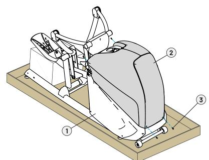
B. Remove and set aside the top shroud assembly.
