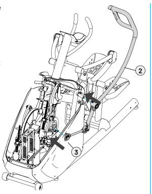
C. Attach the moving handlebar to the shaft with an M10 washer and M10 bolt.
