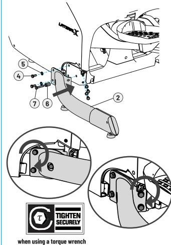
E. Using a #2 Phillips screwdriver and #2 Phillips stubby screwdriver attach the right stabilizer cover with two M5 screws.
