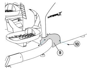
F. Using a #2 Phillips screwdriver and #2 Phillips stubby screwdriver attach the left stabilizer cover with two M5 screws.
