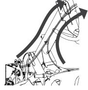
**NOTE:** If needed, use the previously removed wire ties as fishing wire to help pull the cable bundle up and out the top of the mast.
