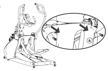
C. Position the top tray shroud over the base frame and around the console mast. Using a #2 Phillips screwdriver, fasten to the frame using two M5 screws from the hardware pack, and then fasten to the back shroud using the two previously removed M5 screws.
