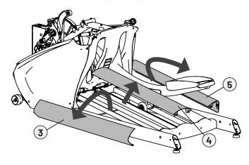
B. Remove any protective coverings and verify the tracks and wheels are clean and free from debris.
