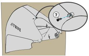
Position the shroud assembly on base frame. Insert and tighten four M5 screws to secure the shrouds in place.
