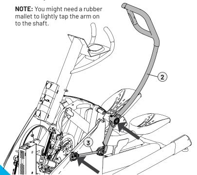
C. Attach the moving handlebar to the shaft with an M10 washer and M10 bolt. Attach the moving arm link to the small crank arm with an M10 nut. Securely fasten all hardware. When using a torque wrench fasten to 45 n-m (33 ft-lb).
