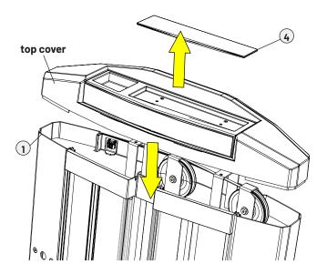
C. Using a 3/32" allen wrench, remove and set aside the 4 tray cover hex screws. Remove and set aside the tray cover.
