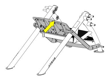
B. Wipe all dirt and dust from the main frame shafts before lightly applying the assembly lubricant. Apply the lubricant to a cloth or paper towel and use it to wipe down the shafts on each side.
