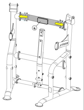
D. When all 12 socket head cap screws and lock washers are finger tight, use a 3/8" allen wrench to fully tighten.
