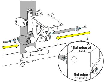
C. Apply Loctite<sup>®</sup> to the bottom shoulder screw and using a 5/32" allen wrench, attach the gas shock to the seat frame assembly.
