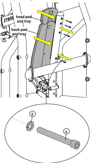
B. Using a 5/16" allen wrench, attach the three socket head cap screws, lock washers, and flat washers to secure the seat pad assembly to the seat frame assembly.
