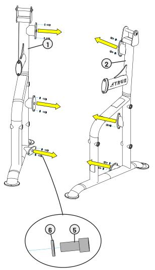
B. Using two people, carefully line up the right and left frame assemblies with the seat frame assembly and finger tight the previously removed socket head cap screws and lock washers.
