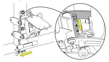
D. Line up flat edge of the upper axle with the flat edge of the frame/shaft. If needed, use a rubber mallet to lightly tap the axle into the shaft. Apply Loctite<sup>®</sup> to the two socket head cap screws, and using a 5/16" allen wrench, attach the socket head cap screws, lock washers, and caps to the upper side plates and seat frame assembly.
