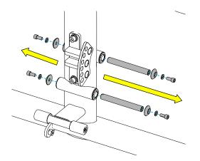
B. Line up flat edge of the lower axle with the flat edge of the frame/shaft. If needed, use a rubber mallet to lightly tap the axle into the shaft. Apply Loctite<sup>®</sup> to the two socket head cap screws, and using a 5/16" allen wrench, attach the socket head cap screws, lock washers, and caps to the lower side plates and seat frame assembly.
