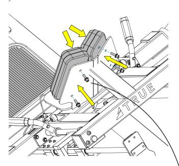
B. Using a 5/16" allen wrench, attach the three socket head cap screws, lock washers, and flat washers to secure the seat pad assembly to the seat frame assembly.
