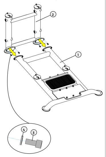
2. Using two people, carefully line up the rear frame assembly with the base assembly and finger tight the previously removed socket head cap screws and lock washers. DO NOT fully tighten until the left and right rail frame pieces have also been aligned and finger tightened.
