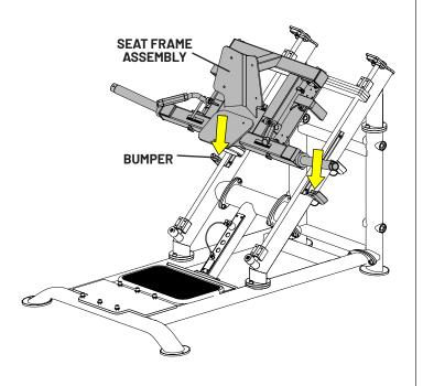
D. Using at least two people, remove the wooden alignment piece and slide the bearing assemblies underneath the attachment points of the seat frame assembly.
