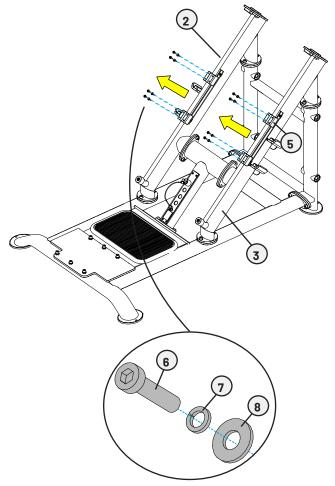
**ACAUTION:** DO NOT remove the linear bearings assemblies (D 312M) from the rails and try to attach them to the seat frame assembly. The bearings will not slide back onto the rails with the seat attached.
