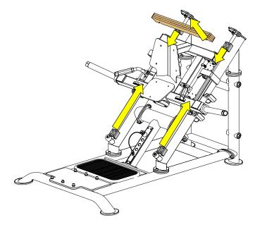
E. Using at least two people, carefully fasten the seat frame assembly to the bearing assemblies using the previously removed socket head cap screws, lock washers, and flat washers. Once all the hardware is finger tight, use a 3/16" ball end allen wrench to fully tighten.
