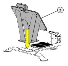
C. Align the holes of the base frame assembly with the holes of the foot plate assembly and then finger tighten the six previously removed socket head cap screws, lock washers, and flat washers.
