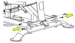
E. When all four socket head cap screws, lock washers, and flat washers are finger tight, use a 5/16" allen wrench to fully tighten.
