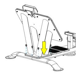
D. When all six socket head cap screws, lock washers, and flat washers are finger tight, use a 3/8" allen wrench to fully tighten.
