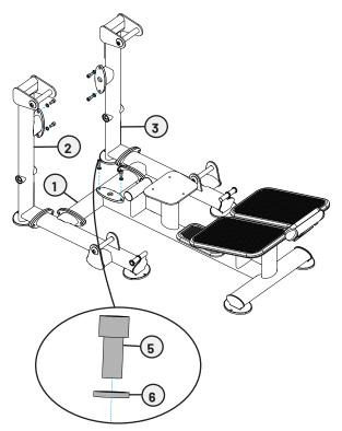
B. Using two people, carefully line up the seat pad support assembly with the base frame assembly and right and left rear main frame assemblies and finger tighten the previously removed socket head cap screws and lock washers.
