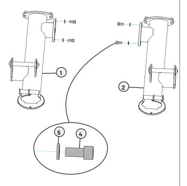
B. Using two people, carefully line up the right and left side base frame assemblies with the base frame assembly and finger tighten the previously removed socket head cap screws and lock washers.
