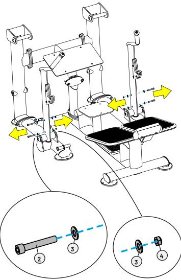
B. Using two people, carefully line up the cross brace assembly with the right and left stop arm assemblies and finger tighten the previously removed socket head cap screws, flat washers, and lock nuts.
