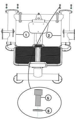
B. Using two people, carefully line up the right and left side base frame assemblies with the right and left rear main frame assemblies and finger tighten the previously removed socket head cap screws and lock washers.
