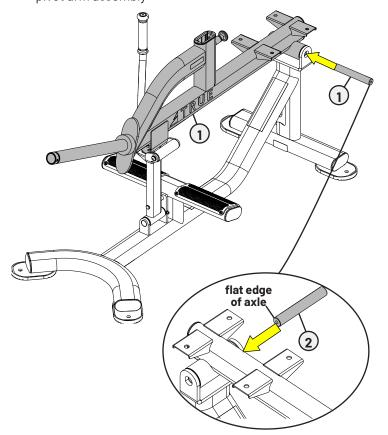
C. Using a 7/32" allen wrench, attach the pivot arm assembly to the top of the main frame assembly using 2 hex screws and 2 aluminum caps.
