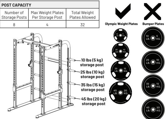
**IMPORTANT!** Storage posts are 50 mm in diameter, designed to accommodate olympic weight plates with center hole diameters of 50 mm. Spacing between the storage posts is specific to olympic weight plates and will not accommodate bumper plates.
