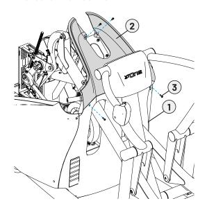
B. Slide the console mast over the four screws on the base. Using a 6mm allen wrench, securely fasten the hardware.
