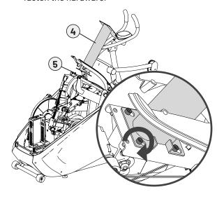
C. Remove the wire ties securing the cable bundle under the mast. Route the cable bundle up and out the top of the mast.
