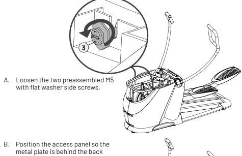
side screws and then secure the access panel and back shroud with two M5 screws.
