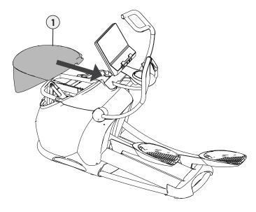
B. Fasten the top shroud to the access panel with two M5 with flat washer screws.
