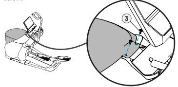
C. Wrap the mast boot around the console mast and tuck into access panel.
