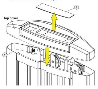
C. Using a 3/32" allen wrench, remove and set aside the 4 tray cover hex screws. Remove and set aside the tray cover.
