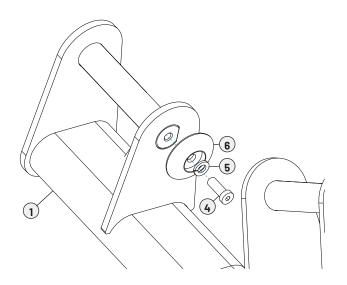
B. With the outside caps, hex screws, and lock washers still attached, use a rubber mallet to remove the 2 axles.
