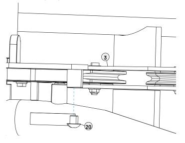
N. Using a ball end allen wrench, reattach the 1 hex screw you removed previously.
