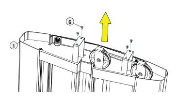
B. Place the top cover onto the upright assembly. Remove and set aside the tray mat.
