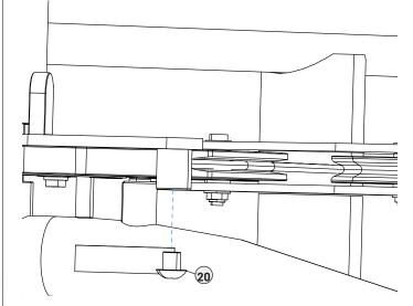
M. Route the main frame cable around the pulleys and pulley cam and fasten it into place.
