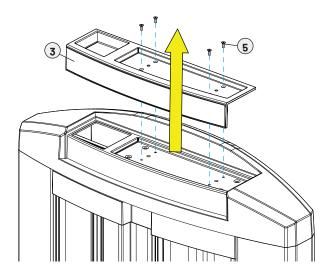
D. Attach the top cover to the upright assembly using the 4 previously set aside top cover hex screws.
