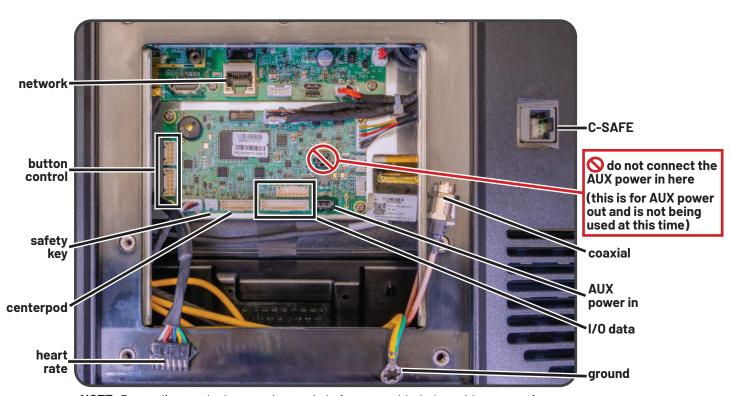
**NOTE:** Depending on the base and console being assembled, the cable connections will vary. Examples of the cable ports and connections are shown above. See the base assembly manual for the specific cable connections being made.
