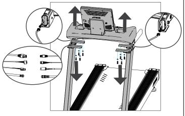
f. Using a 5mm allen wrench, remove and set aside the four hex screws securing the handrail assembly to the pedestal assemblies.
