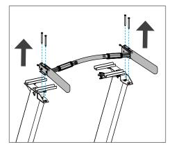
2. Using a 6mm allen wrench, remove the two hex screws and washers securing the left and right handrails to the contact heart rate bar.
