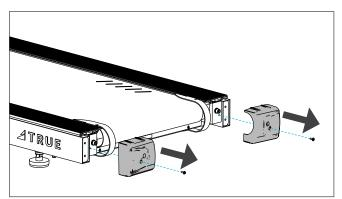
4. Using a #2 Phillips screwdriver and the two previously set aside screws, secure the extended handrail left and right rear roller covers to the frame.
