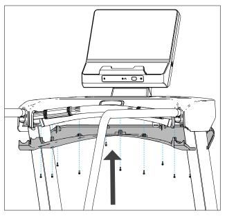
9. Using a #2 Phillips screwdriver, attach the left and right extended handrail covers.
