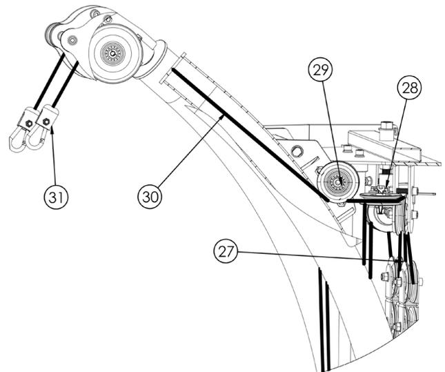
MINIMUM INSERTION LENGTH OF 0.5" (12.7mm) OF TOP FRAME ASSEMBLY BOLT INTO ADJUSTABLE TOP PULLEY HOUSING.
