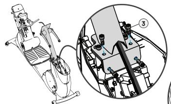
C. Using a 6mm allen wrench, securely fasten all six M8 hex screws. When using a torque wrench fasten to 40 n-m (30 ft-lb).
