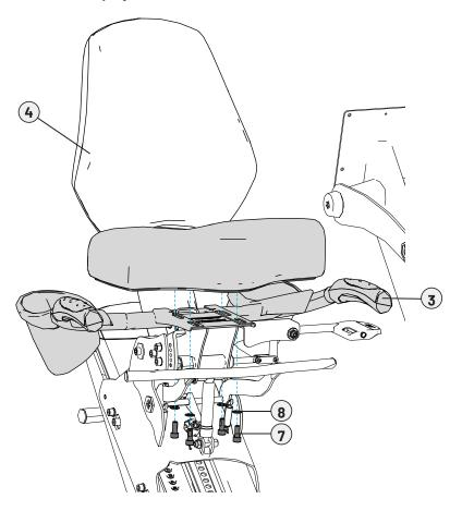
F. Tilt the seat forward so you can attach the tilt control cable. Place the tilt control cable into the hole on seat carriage and slide up to secure in place.
