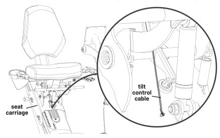
G. Using a 6mm hex wrench and 13mm wrench remove and set aside the M8 hex screw, washers, and nut from the bracket on the seat carriage.
