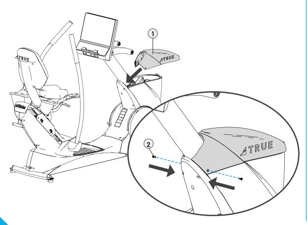
B. Wrap the mast boot around the console mast.
