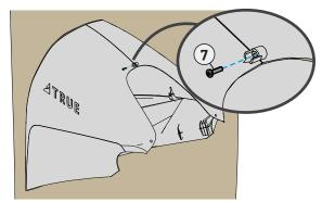
Position the shroud assembly on base frame.
