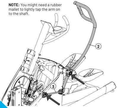
C. Attach the moving handlebar to the shaft with an M10 washer and M10 bolt. Attach the moving arm link to the small crank arm with an M10 nut.
