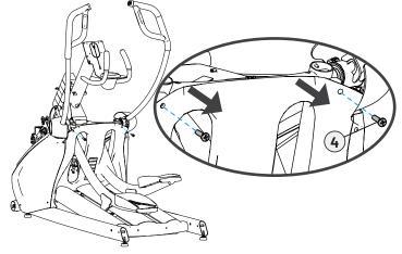
C. Position the top tray shroud over the base frame and around the console mast. Using a #2 Phillips screwdriver, fasten to the frame using two M5 screws from the hardware pack, and then fasten to the back shroud using the two previously removed M5 screws.
