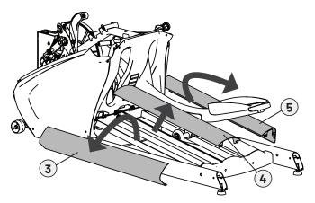
B. Remove any protective coverings and verify the tracks and wheels are clean and free from debris.
