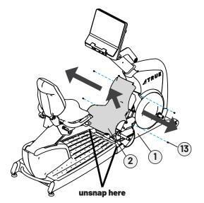
B. Using a #2 Phillips screwdriver on both sides of the machine, remove and set aside the screws securing the crank arm covers and them remove and set aside the covers.
