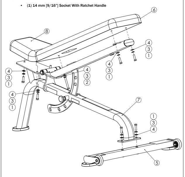
Verify that the back pad and seat pad frames can easily be adjusted to each position. Verify that the adjustment pin is fully inserted during each adjustment.
