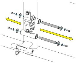
B. Line up flat edge of the lower axle with the flat edge of the frame/shaft. If needed, use a rubber mallet to lightly tap the axle into the shaft. Apply Loctite® to the two socket head cap screws, and using a 5/16" allen wrench, attach the socket head cap screws, lock washers, and caps to the lower side plates and seat frame assembly.
