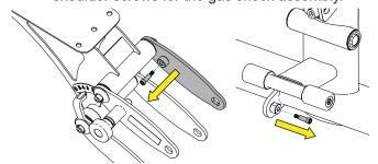
b. Using a 5/16" allen wrench, remove the socket head cap screws, lock washers, and caps securing the upper and lower axles to the seat frame.
