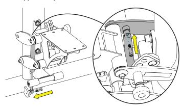
D. Line up flat edge of the upper axle with the flat edge of the frame/shaft. If needed, use a rubber mallet to lightly tap the axle into the shaft. Apply Loctite® to the two socket head cap screws, and using a 5/16" allen wrench, attach the socket head cap screws, lock washers, and caps to the upper side plates and seat frame assembly.
