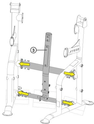
**NOTE:** As you align the parts together, it helps to use the styrofoam from the packaging to place under the frame pieces.
