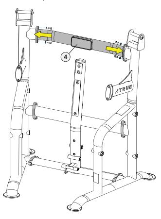
D. When all 12 socket head cap screws and lock washers are finger tight, use a 3/8" allen wrench to fully tighten.
