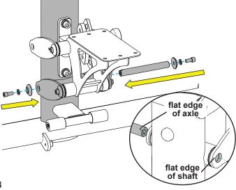
C. Apply Loctite® to the bottom shoulder screw and using a 5/32" allen wrench, attach the gas shock to the seat frame assembly.
