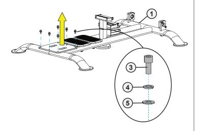
B. Using three people, carefully place the foot plate assembly onto the base frame assembly.
