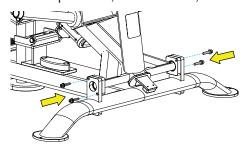
E. When all four socket head cap screws, lock washers, and flat washers are finger tight, use a 5/16" allen wrench to fully tighten.
