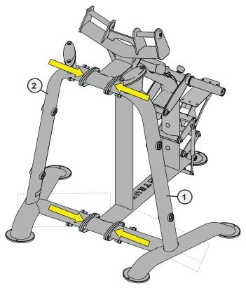
**NOTE:** As you align the parts together, it helps to use the styrofoam from the packaging to place under the frame pieces.
