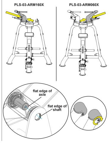
A. Using a 5/16" allen wrench, remove and set aside the socket head cap screws, lock washers, caps, and axles from the right and left frame assemblies.
