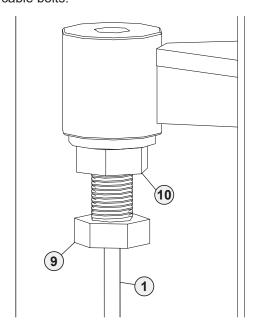
**IMPORTANT!** A minimum of ½" (12.7mm) of the threaded portion of the cable bolt must be threaded into the cable attachment point. Make sure locking nut is tight.
