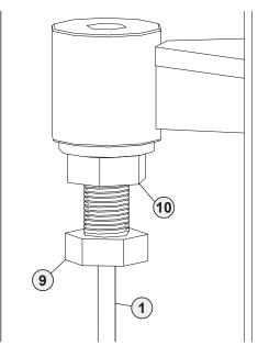
**IMPORTANT!** A minimum of ½" (12.7mm) of the threaded portion of the cable bolt must be threaded into the cable attachment point. Make sure locking nut is tight.
