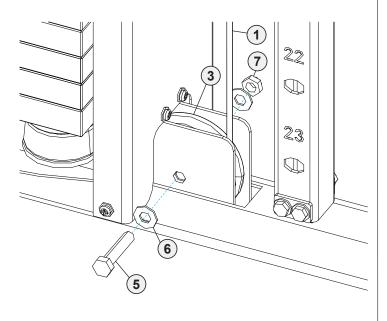
K. Attach the cables to the cable attachment points using the cable bolts.
