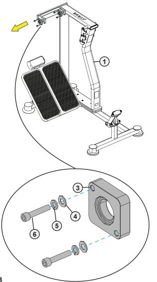
B. Using three or more people, carefully slide one bearing assembly onto the lifting arm assembly and then place the lifting arm assembly into the side frame assembly.
