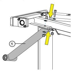
C. Using a 5/16" allen wrench, remove and set aside the socket head cap screw, lock washer, and cap from the counter weight post assembly.
