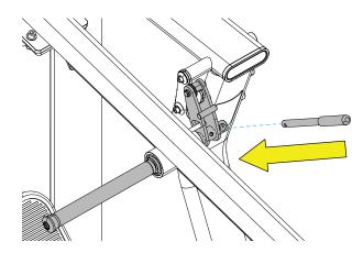
D. Attach the catch assembly and catch assist assembly to the handle bar using the shoulder screw, socket head cap screw, lock washer, flat washers, and nut.
