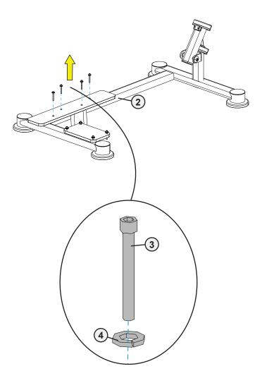
B. Using three or more people, carefully line up the side frame assembly with the base frame assembly and finger tight the previously removed socket head cap screws and lock washers.
