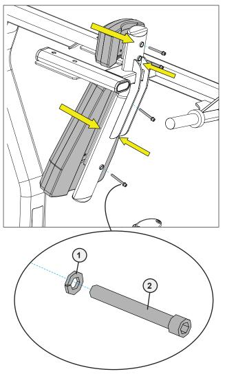
B. Using a 5/16" allen wrench, attach the four socket head cap screws and sleeves to secure the shoulder pads to the lifting arm assembly.
