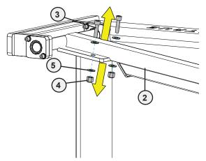
B. Using two people, carefully attach the counter weight assembly to the lifting arm assembly and secure in place using the previously removed socket head cap screws, flat washers, and nuts.
