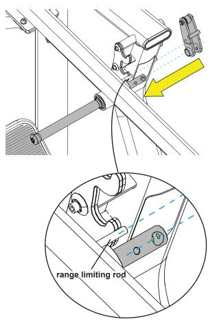
C. Slide the catch assist assembly into the hole of the handle bar.
