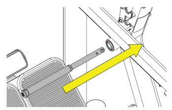
B. Slide the catch assembly onto the handle bar and align with range limiting rod on the lifting arm assembly.
