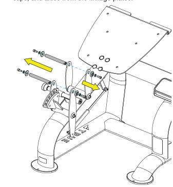
C. Using two people line up the seat back assembly with the linkage plates and secure in place using the previously removed axles, caps, lock washers, and socket head cap screws. Once all the pieces are lined up and finger tight, use a 5/16" and 5/32" allen wrench to verify all seat assembly and gas shock hardware is fully tightened.
