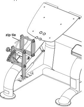
B. Using a 5/16" allen wrench remove and set aside the preinstalled socket head cap screws, lock washers, caps, and axles from the linkage plates.
