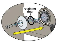
IMPORTANT! Verify the retaining ring is completely wrapped around the end of the leg assembly axle.
