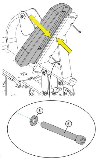
B. Using a 5/16" allen wrench, attach the six socket head cap screws, lock washers, and flat washers to secure the seat pad assemblies to the seat frame assembly.
