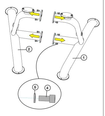
B. Using two people, carefully line up the right and left side frame assemblies with the seat frame assembly and finger tight the previously removed socket head cap screws and lock washers.
