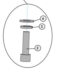
B. Using a 5/16" allen wrench, attach the two socket head cap screws, lock washers, and flat washers to secure the two roller pad assemblies to the center frame assembly.
