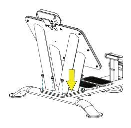
D. When all six socket head cap screws, lock washers, and flat washers are finger tight, use a 3/8" allen wrench to fully tighten.
