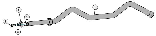
B. Slide the handle bar assembly into the frame and then using a 5/16" allen wrench and retaining ring pliers, attach the retaining ring, cap, lock washer, and socket head cap screw to secure the handle bar assembly to the frame.
