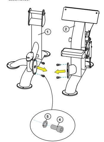
B. Using two people, carefully line up the center cross brace assembly with the two frame assemblies and finger tight the previously removed socket head cap screws and lock washers.
