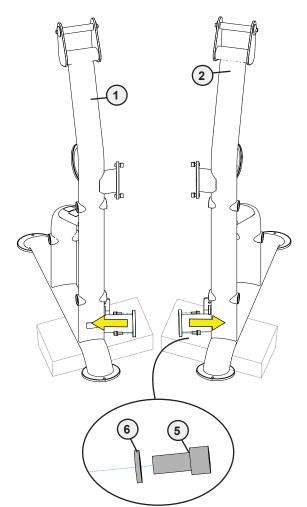
B. Using two people, carefully line up the right and left frame assemblies with the seat frame assembly and finger tight the previously removed socket head cap screws and lock washers.
