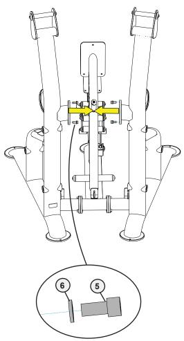
D. Carefully line up the right and left frame assemblies with the cross brace assembly and finger tight the previously removed socket head cap screws and lock washers.
