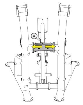
E. Once all the frame pieces have been assembled, use a 3/8" allen wrench to fully tighten.
