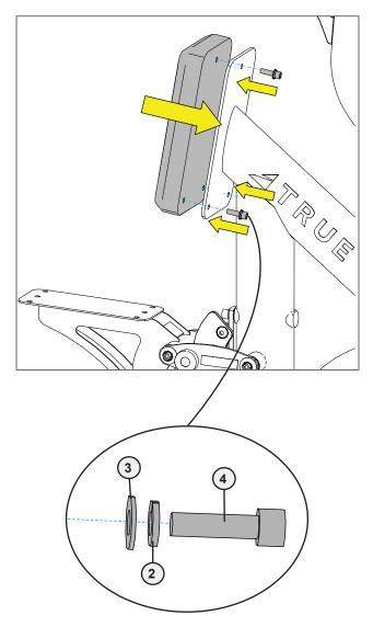
B. Using a 5/16" allen wrench, attach the two socket head cap screws, lock washers, and flat washers to secure the seat pad assembly to the seat frame assembly.
