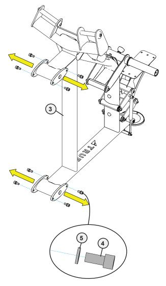
B. Using two people, carefully line up the right and left main frame assemblies with the center assembly and finger tight the previously removed socket head cap screws and lock washers.
