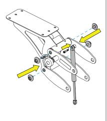
5. Line up flat edge of the axle with the flat edge of the frame/shaft and using a rubber mallet, lightly tap the axle into the shaft. Apply Loctite® to the two socket head cap screws, and using a 5/16" allen wrench, attach the socket head cap screws, lock washers, and caps to the lower side plates and seat frame assembly.
