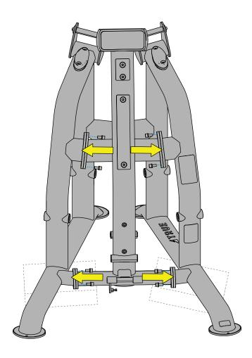
**NOTE:** As you align the parts together, it helps to use the styrofoam from the packaging to place under the frame pieces.
