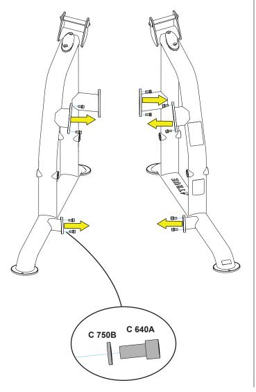
2. Using two people, carefully line up the rear right and left main frame assemblies and finger tight the previously removed socket head cap screws and lock washers.
