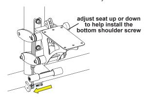
7. Line up flat edge of the axle with the flat edge of the frame/shaft and using a rubber mallet, lightly tap the axle into the shaft. Apply Loctite® to the two socket head cap screws, and using a 5/16" allen wrench, attach the socket head cap screws, lock washers, and caps to the upper side plates and seat frame assembly.
