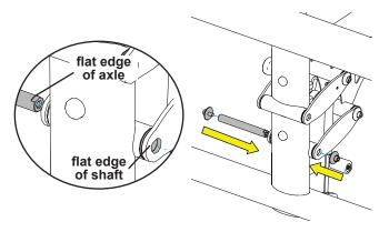
Adjust the seat up or down to help align the gas shock with the lower attachment point. Apply Loctite<sup>®</sup> to the bottom shoulder screw and attach the gas shock to the seat frame assembly.
