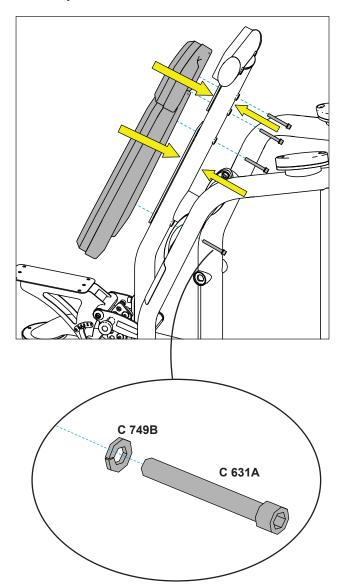
2. Using a 5/16" allen wrench, attach the three socket head cap screws, lock washers, and flat washers to secure the seat pad assembly to the seat frame assembly.
