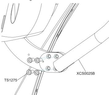
2. Using a #2 Phillips screwdriver, attach the exercise arm covers using 8 screws.
