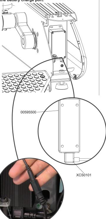
Secure the power supply to the bracket using 2 zip ties.
