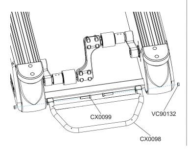
2. Using a #2 Phillips screwdriver, attach the rear step frame cover to the rear step frame using 4 screws.
