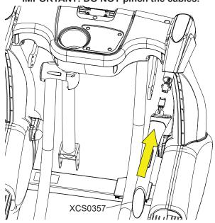
3. Using a 6mm allen wrench, attach the side arms to the pedestal using 4 hex screws.
