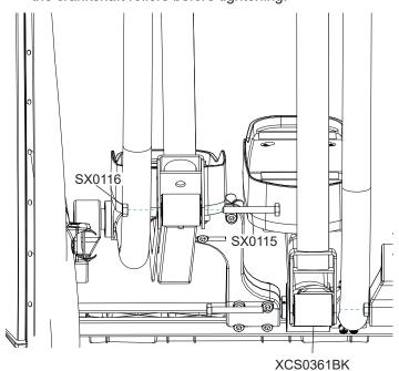
2. Using a #2 Phillips screwdriver, attach the rocker arm covers using 8 screws.
