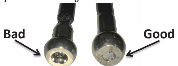
Crimp Connector Dislodged:
