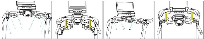
b. Using a 5mm allen wrench, remove and set aside the four screws and washers securing the left and right handrails to the pedestals.
