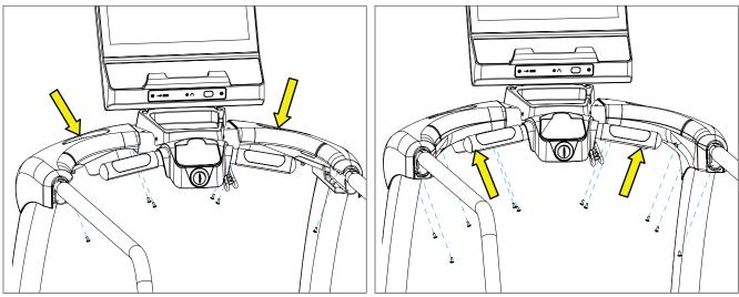
7. Using a #2 Phillips screwdriver, attach the left and right rehab rail clamshell assemblies.
