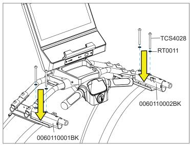
4. Using the two existing rear roller cover screws and a #2 Phillips screwdriver, attach the rehab rail kit end caps to the frame.
